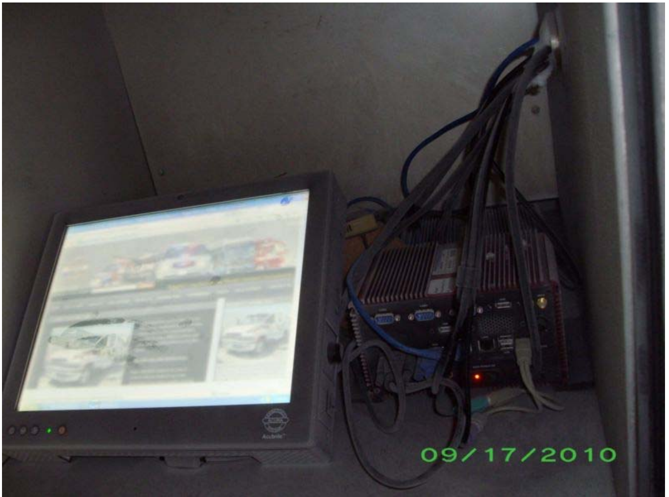
Picture 5 – Low Temperature Test setup inside of Test Chamber
