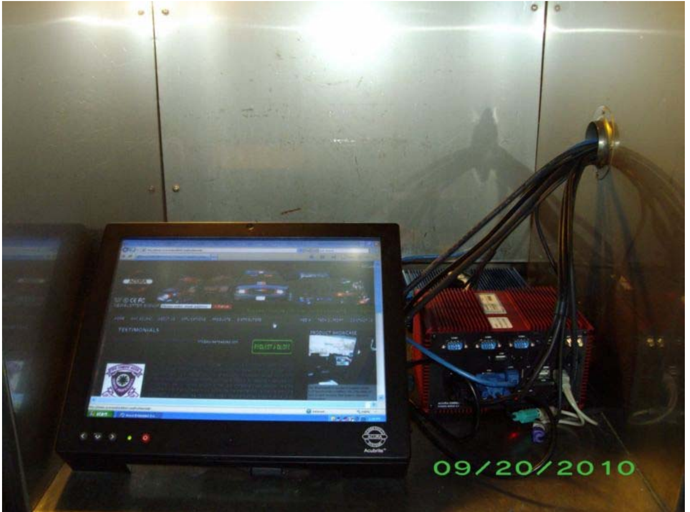
Picture 6 – High Temperature Test Setup inside the Test Chamber
